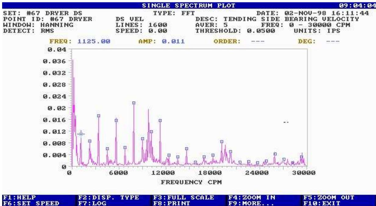
Harmonics of outer race defect frequency (1125 RPM) marked in spectrum. Note outer race defect in photo below.
