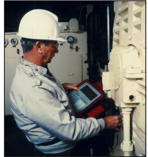
Figure 1. The portable data collector is used to measure casing vibration and shaft motion in displacement, velocity, and acceleration. On a boiler feed pump, for instance, the measurements are taken in three directions – horizontal, vertical, and axial – at each bearing location throughout the entire equipment train.
