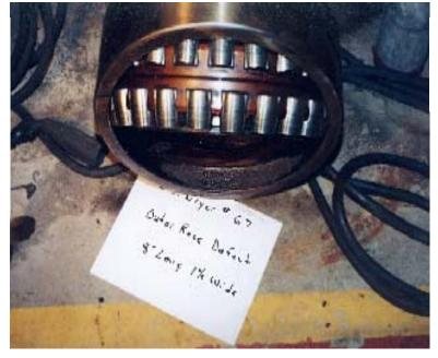
The defects can be seen in this photo at the bottom of the outer race.
