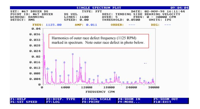
The spectrum above shows harmonics of this bearings outer race defect frequency at 1125 RPM. These frequencies were produced by a defect 8 inches long and  $1\frac{1}{2}$ inches wide.
